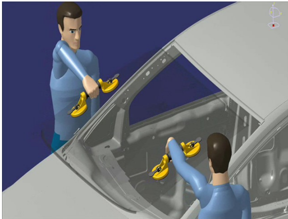
Figure 3: Snapshot from the video showing the process animation of the windshield assembly task.
