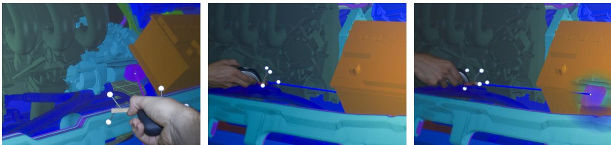
Figure 1: The first two images (a, b) illustrate the issue of interpersonal occlusion between two tracked users in a multi-user VR system: an object that is fully visible to one user (a) cannot or only partially be seen from other viewpoints (b). Show-through techniques can improve target discovery in such situations by showing the indicated object through the occluding environment (c).
