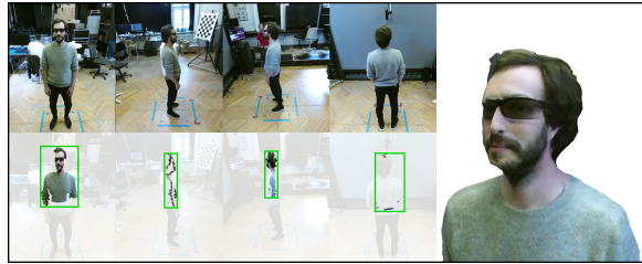
Fig. 9: Example of our pre-blended texture creation. The avatar (right) is seen by a local participant and its lower body is out of frustum. Areas in the input color textures (top row) contributing to visible triangles are blended and stored in the output textures (bottom row). Only texels contained in the tight texture bounding boxes (green) are transmitted to the clients.
