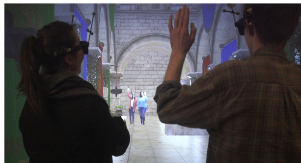
Fig. 10: Our Three-to-Two Scenario: Three collocated telepresence participants meet two remote participants in a shared virtual scene. Due to the size of the multi-user 3D display, the local participants see similar perspectives of the remote participants' 3D video avatars and the scene. Note that the photo camera assumes the role of a third local participant.
