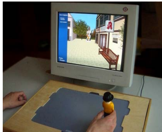
Figure 1: User navigating through the virtual environment by moving a puppet-shaped prop over the board. Actions are initiated by pressing a button in the hat of the prop.
